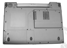
Figure 2-7 Remove the HDD compartment cover
